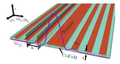
Scheme of considered structure. A periodically repeated supercell consisting of a = 100 nm wide (x-direction) and t = 6 nm thick 43 elementary cells. On the 50% of the top and bottom surfaces of each elementary cell (except the defect) surface anisotropy was applied-see red area. The strength of surface anisotropy was determined by the surface anisotropy constant. For the sake of symmetry, the defect was placed at the center of the supercell.
